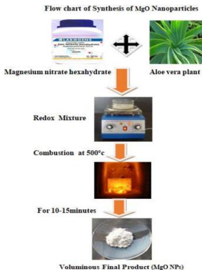
Fig 3: Flow chart for preparation of MgO nanoparticles
