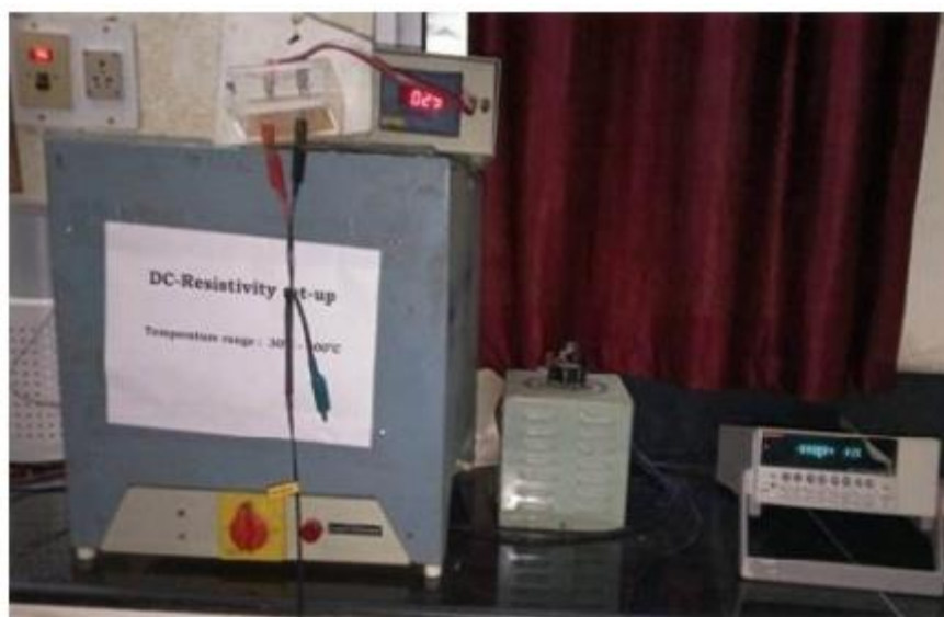
Fig3.19: Experimental set-up for DC conductivity measurements
