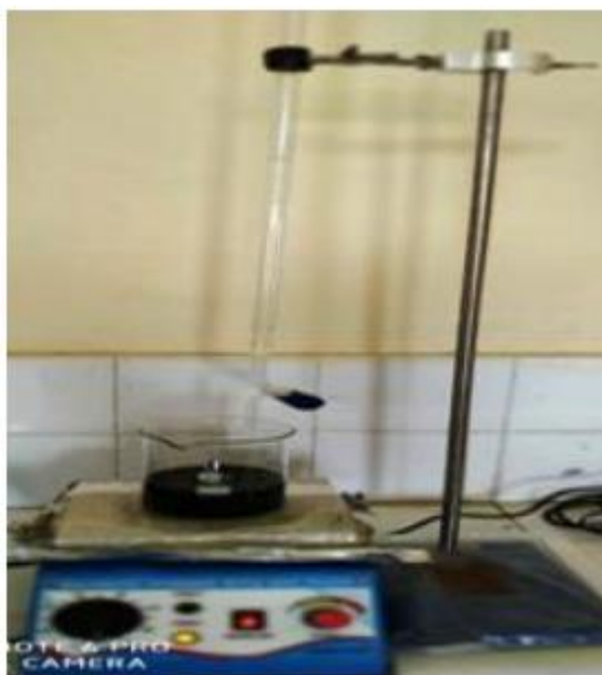
Fig 1: A photograph for solution mixing using magnetic stirrer
